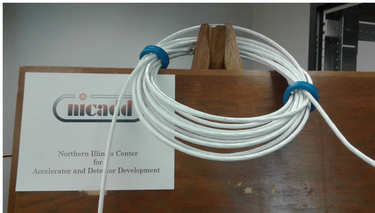
FIGURE 4.9: An image of the SSP cable configuration. The 30 foot cable is looped through two magnetic cores and oriented to reduce its ability to act as a radio antenna.
