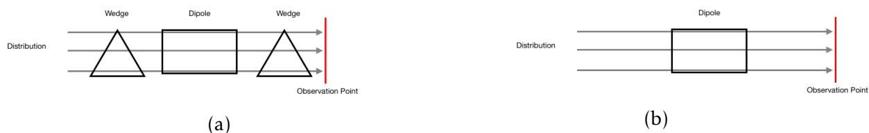
Figure 4.20: One simulation will be run with wedges in the lattice, (a), and compared to a run with the wedges removed from the lattice, (b). The observation point is where the spin in each of these two cases will be examined.
